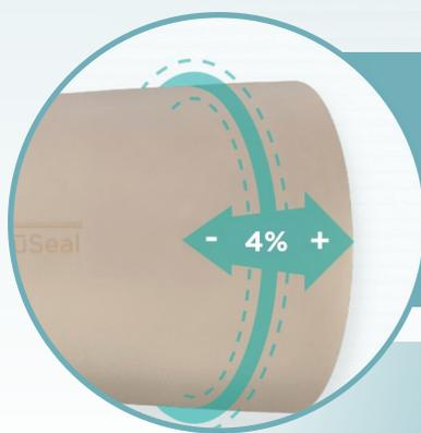
Silicone Volume Management Pads (VMPs) accommodate up to 8% range of volume fluctuation.
